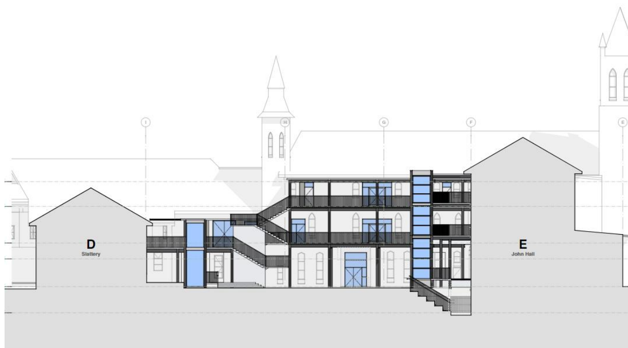
Figure 6.1: Proposed Quadrangle Elevation showing the new steel-framed walkways, stairs and lift against the rear elevation of the main buildings of the school. (not to scale)
